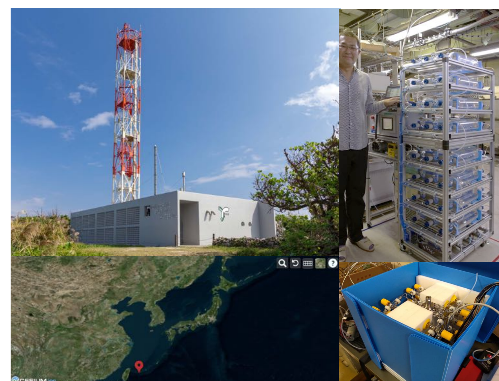
Figure 5. (Left top) A picture of the Hateruma Station (HAT), Japan ( https://esd.nies.go.jp/a/about/facilities/ ). (Left bottom) Location of HAT (red icon, https://db.cger.nies.go.jp/ged/ ). (Right top) A picture of the Hateruma event sampler (HEV). This sampler collects sample air into series of ~2.5 L glass flasks at pre-scheduled timings. (Right bottom) A picture of the compact air sampler (CASPER). This sampler houses series of ~0.1 L glass flasks. The sampler switches automatically and post-decision samplings are made, referring to in-situ CH 4 measurement.
